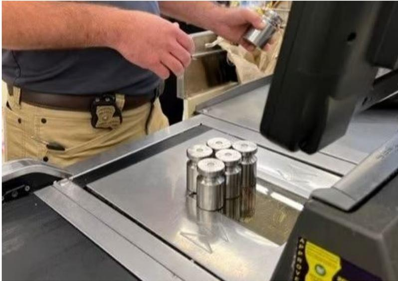
Weighmaster testing scale
